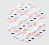
It is ideal for high and medium power applications and the most commonly used LED assembling purposes from 1W to 2W. Highly recommended for mass production with cost restrictions.
